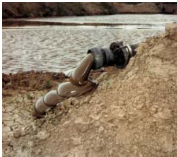
Abrasive sludges with a high concentration of solid mater can be transported without problem.
